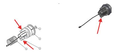
3. Place the new plunger in the hole from the top and (with the spring threaded through the cable) and connect the new cable to the existing cable.
